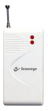
This is the perimeter protection for the wall or glass or and other buildings. The vibration sensor is usually installed on doors and windows and walls. The vibration sensor operates on the principle that when the door or window or walls vibrated by the intruder shock or dig, will trigger a signal to alarm system. The vibration sensor is popular and widely used because they detect an intruder before he enters the protected premises.
