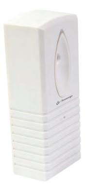
This is the perimeter protection for the wall or glass or and other buildings. The vibration sensor is usually installed on doors and windows and walls. The vibration sensor operates on the principle that when the door or window or walls vibrated by the intruder shock or dig, will trigger a signal to alarm system. The vibration sensor is popular and widely used because they detect an intruder before he enters the protected premises.
