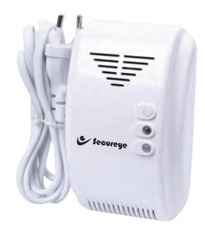
The Wireless Gas Leakage Detector is an input device designed for natural gas, LPG detection. It can use independently or as a front-end detector of an alarm system. Upon detection of natural gas and LPG, this device automatically generates an alarm signal to control panel and sound & flash alarm.
