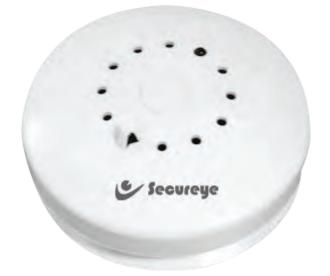
The Compound Temperature Sensor is special for normally temperature and smoke detect applications, e.g.: Facotry, Laboratory, museum, warehouse, wareroom, storehouse, depot, depository, depositary, generator room, machine room, engine room, etc. If it detected the temperature higher than 70°C or there're heavy smoke, the detector will trigger and output one dry contact singal to the alarm system (if wired sensor, only work with S3523, S3526). The alarm system will alert the users immediately.
